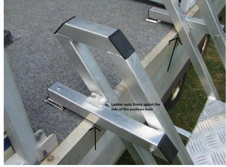
• Next, place the two stainless steel locking keyhole brackets on the ladder nipples and note position on the pontoon deck. Ensure that the ladder is firm against pontoon boat side. See picture of an installed ladder below:
